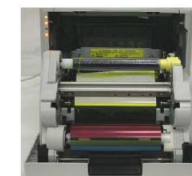
removing the ribbon cassette
