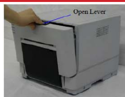
opening the printer
