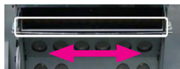
cleaning the thermal head
