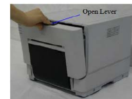
opening the printer
