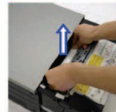
4. Remove the scrap box and rewind the paper. Cut off any partially printed, wrinkled or otherwise inferior paper evenly with scissors.
