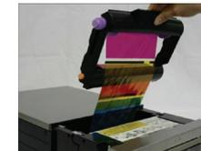
3. Cut the ribbon. Carefully remove any remaining ribbon from inside the mechanism.
