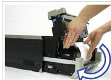
10. Replace the scrap bin, and close the top of the mechanism unit.
